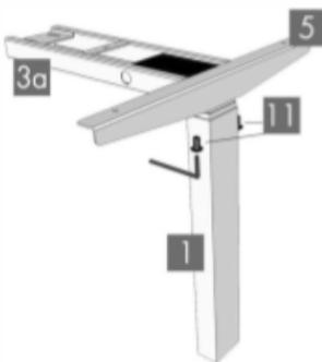
The Frame End-CB (part 3a) should be placed on the side of the desk where you plan to mount the Control Box (part 6) and the Handset (part 7).
